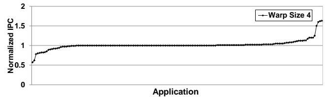
(a) Performance of 165 real world applications using a warp size of 4, normalized to a warp size of 32.
